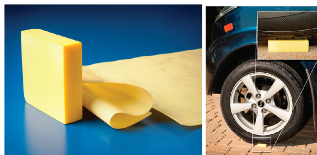
Figure 2. (a) Polyimide aerogels cross-linked with TAB shown fabricated as flexible thin films or molded to a net shape, and (b) demonstrating strength by supporting the weight of a car.
